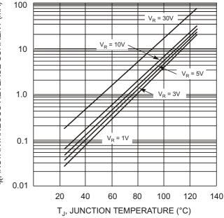
Fig. 2, Typical Pulsed Reverse Characteristics
