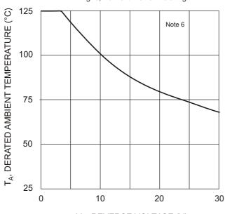
$V_R$ , REVERSE VOLTAGE (V) Fig. 7 Operating Temperature Derating
