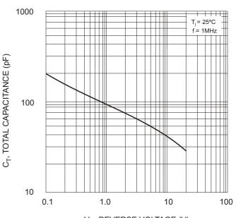
V<sub>R</sub>, REVERSE VOLTAGE (V) Fig. 4, Typical Total Capacitance vs. Reverse Voltage
