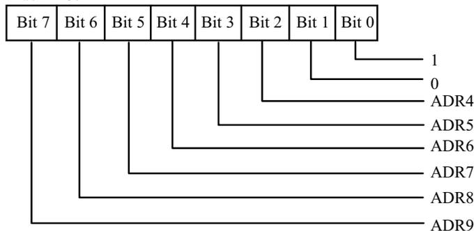
This register is used to select the base address of the IDE Interface Alternate Status Registers.
