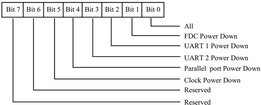
This register controls which part falls in power down mode.
