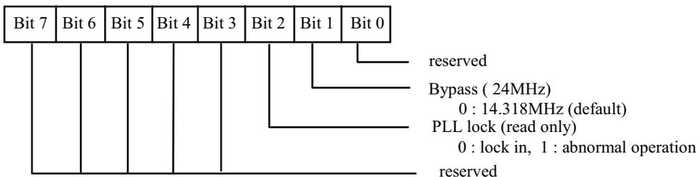
This register controls the operating mode of the clock generator. If you want to use 24MHz external clock, you must change bit 1 of this register . Default = 0 (14.MHz clock)
