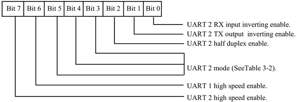
This register controls the operating mode of the UART.
