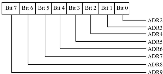
This register is used to select the base address of the parallel port.
