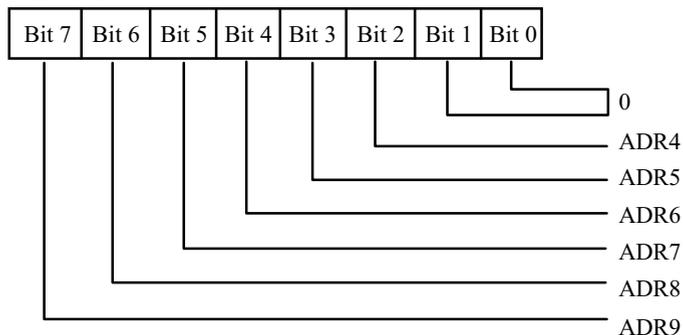
This register is used to select the base address of the IDE Interface Control Registers (0-7).
