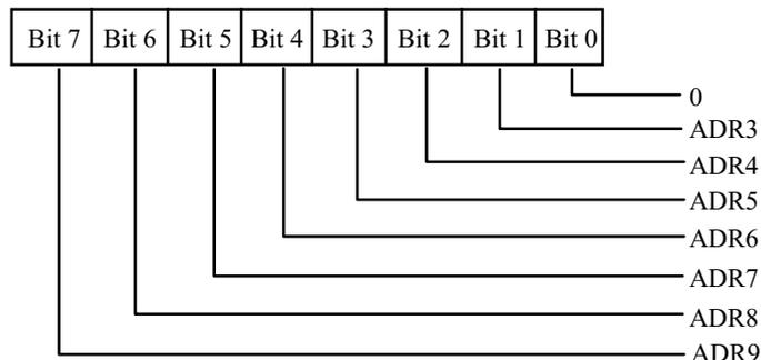
This register is used to select the base address of the UART2.
