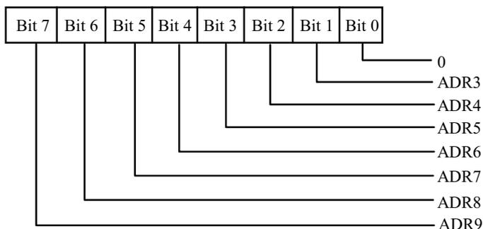
This register is used to select the base address of the UART1.
