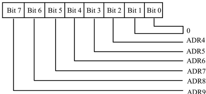
This register is used to select the base address of the Floppy Disk Controller.
