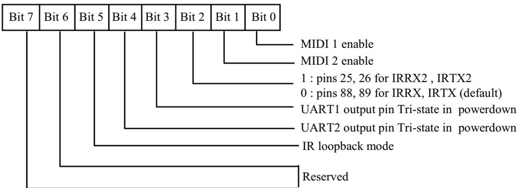
MIDI enable means UART clock is 24 MHz/12 instead of 24 MHz/13
