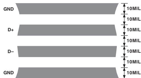
Figure 4. Arrangement of Signal Tracks
