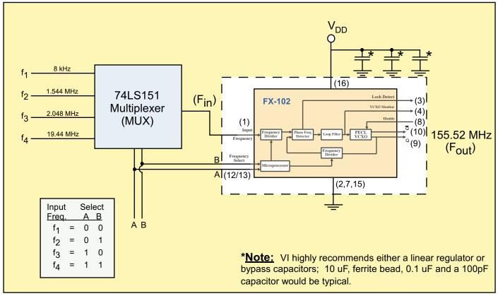
All components outside the dotted line box are user supplied components and/or connections. This is just one possible configuration of the FX-102. For additional information about your specific needs please contact our Factory.
