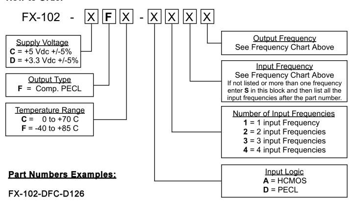
FX-102-DFF-A4S6 - 8 kHz, 1.544MHz, 2.048MHz, 19.44MHz
