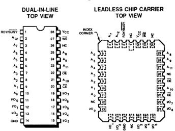
NOTE: The PLCC has the same pin configuration as the LCC except pins 1 and 17 are don't connects.
