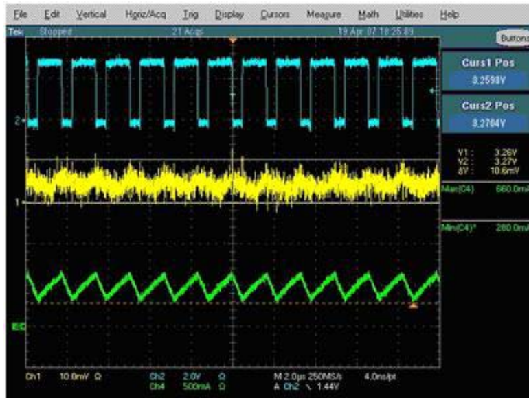
Figure 13. Ceramic 22µF 1210 (X5R) (Good)
