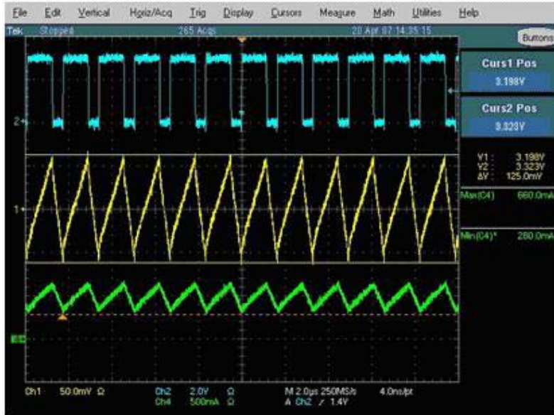
Figure 15. Electrolytic 100 \mu F (Ripple Too High)
