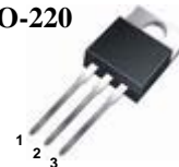
1.Gate 2. Drain 3. Source
