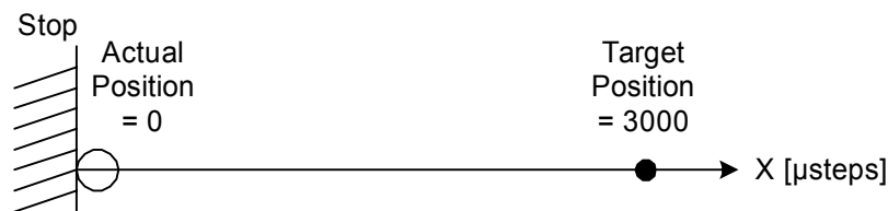
Figure 19: Positioning Example: Situation after reference search
