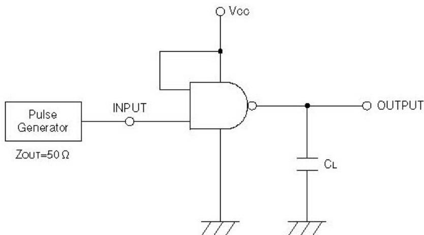
Note: Open output when measuring supply current
