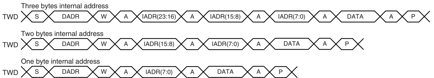
Figure 32-5. Master Write with One, Two or Three Bytes Internal Address and One Data Byte
