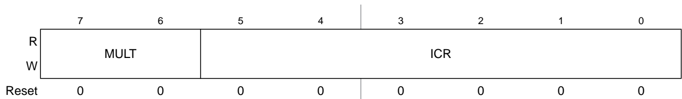
Figure 13-4. IIC Frequency Divider Register (IIC1F)
