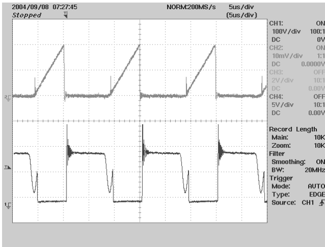
Figure 10 - 85 VAC, Full Load. Upper: I_{DRAIN} , 0.5 A / div Lower: V_{DRAIN} , 100 V, 5 \mu s / div
