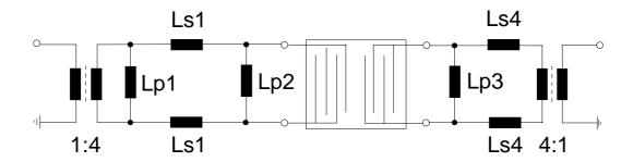
$\begin{aligned} L_{s1} &= 100 \text{ nH} & L_{p3} &= 150 \text{ nH} \\ L_{p2} &= 100 \text{ nH} & L_{s4} &= 150 \text{ nH} \\ L_{p1} &= 560 \text{ nH (for trimming)} \end{aligned}$
