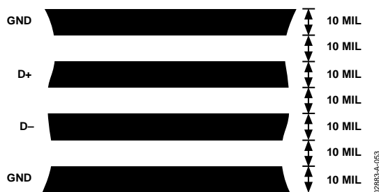
Figure 54. Arrangement of Signal Tracks
