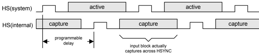
**Figure 15. HSYNC Delay**
