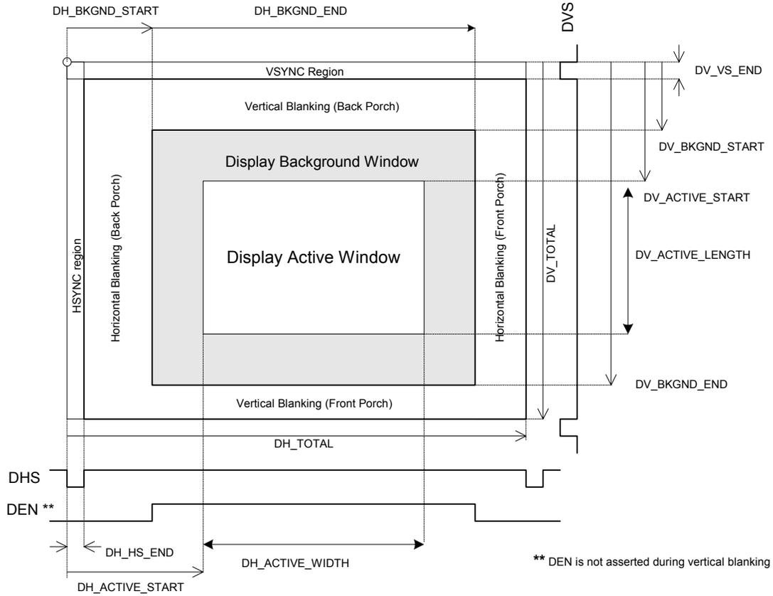
**Figure 19. Display Windows and Timing**
