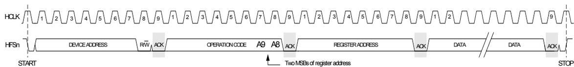
**Figure 30. 2-Wire Write Operations (0x1x & 0x2x)**
