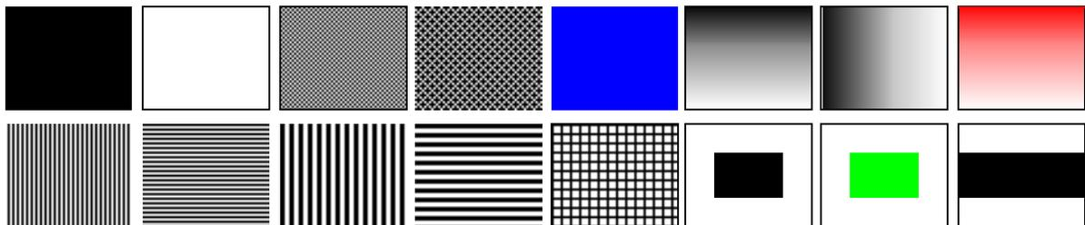
Figure 13. Some of gm5115/25 built-in test patterns
