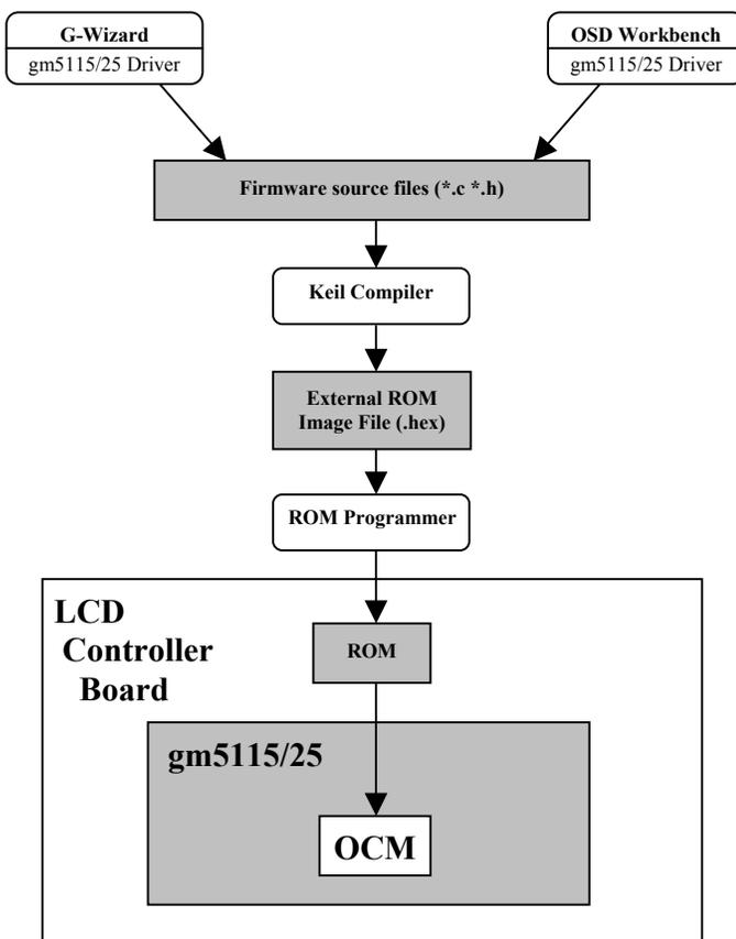
**Figure 28. Programming the OCM in Full-Custom Configuration**
