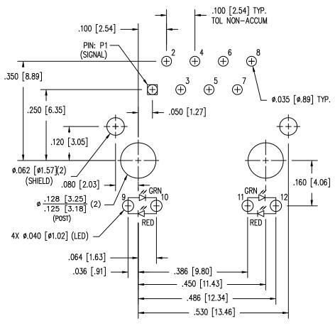
P.C.B. RECOMMENDED HOLE LAYOUT SEEN FROM COMPONENT SIDE TOLERANCE ±.003 [0.08] UNLESS OTHERWISE SPECIFIED (SCALE 4=1)
