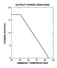
Typical Performance: (Tc=25°C, Vin=Nom VDC, Rated Load)
