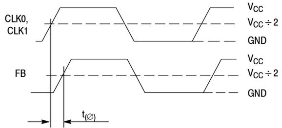
Figure 13. Propagation delay ( $t_{(O)}$ , static phase offset) test reference
