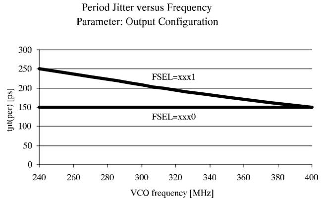
**Figure 7. Max. Period Jitter versus VCO Frequency**
