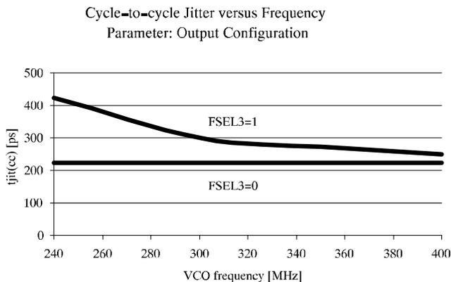
**Figure 6. Max. Cycle-to-Cycle Jitter versus VCO Frequency**
