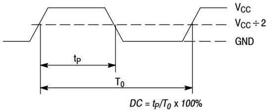
The time from the PLL controlled edge to the non controlled edge, divided by the time between PLL controlled edges, expressed as a percentage
