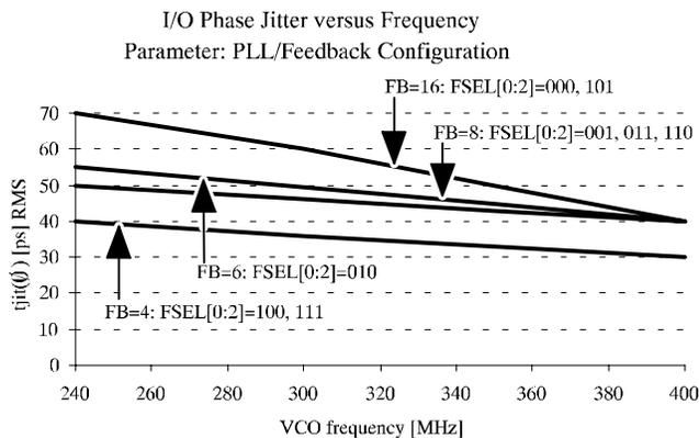
**Figure 5. Max. I/O Phase Jitter versus VCO Frequency**
