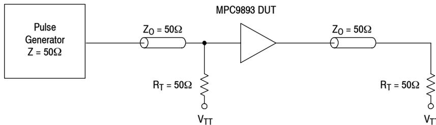
Figure 11. CLK0, CLK1 MPC9893 AC test reference for V<sub>cc</sub> = 3.3V and V<sub>cc</sub> = 2.5V
