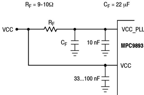
Figure 3. VCC\_PLL Power Supply Filter
