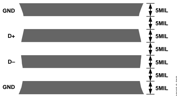
Figure 24. Typical Arrangement of Signal Tracks
