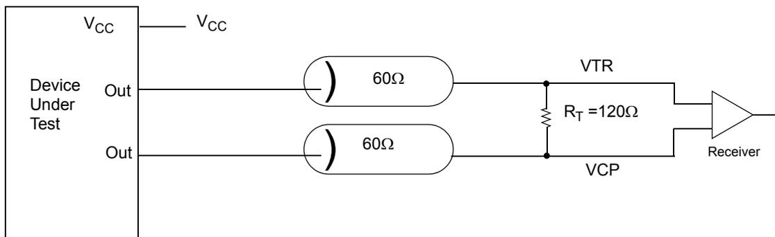
**Figure 1. Differential Signal Using Direct Termination Resistor**
