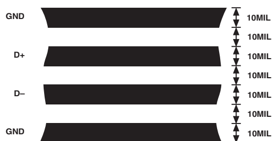
Figure 6. Arrangement of Signal Tracks
