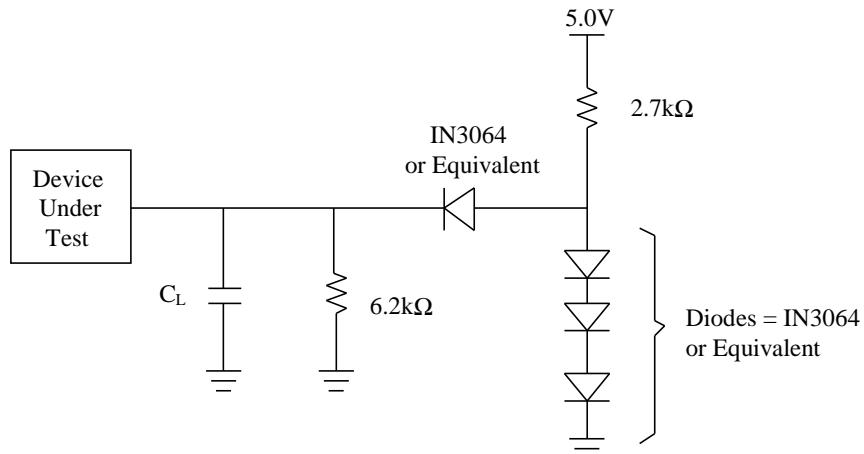
Note :  $C_L = 100\text{pF}$  including jig capacitance
