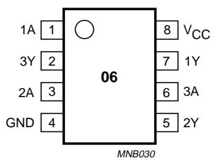
Fig.1 Pin configuration.
