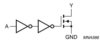
Fig.4 Logic diagram (one driver).
