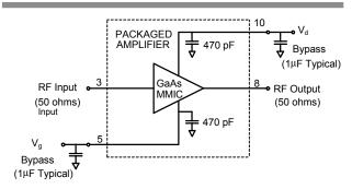
External Components Required: Bypass Capacitors: 1µ F, typical 50 Ohm microsrtip interface
