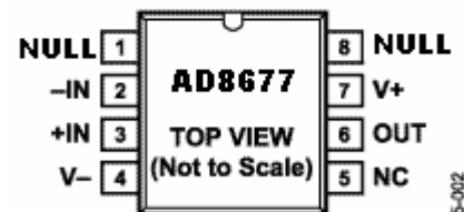
8-Lead SOIC (R-8)
