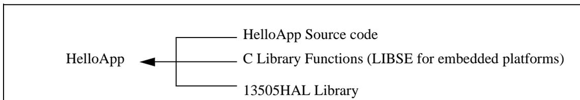
Figure 11-1: Components needed to build 13505 HAL application
