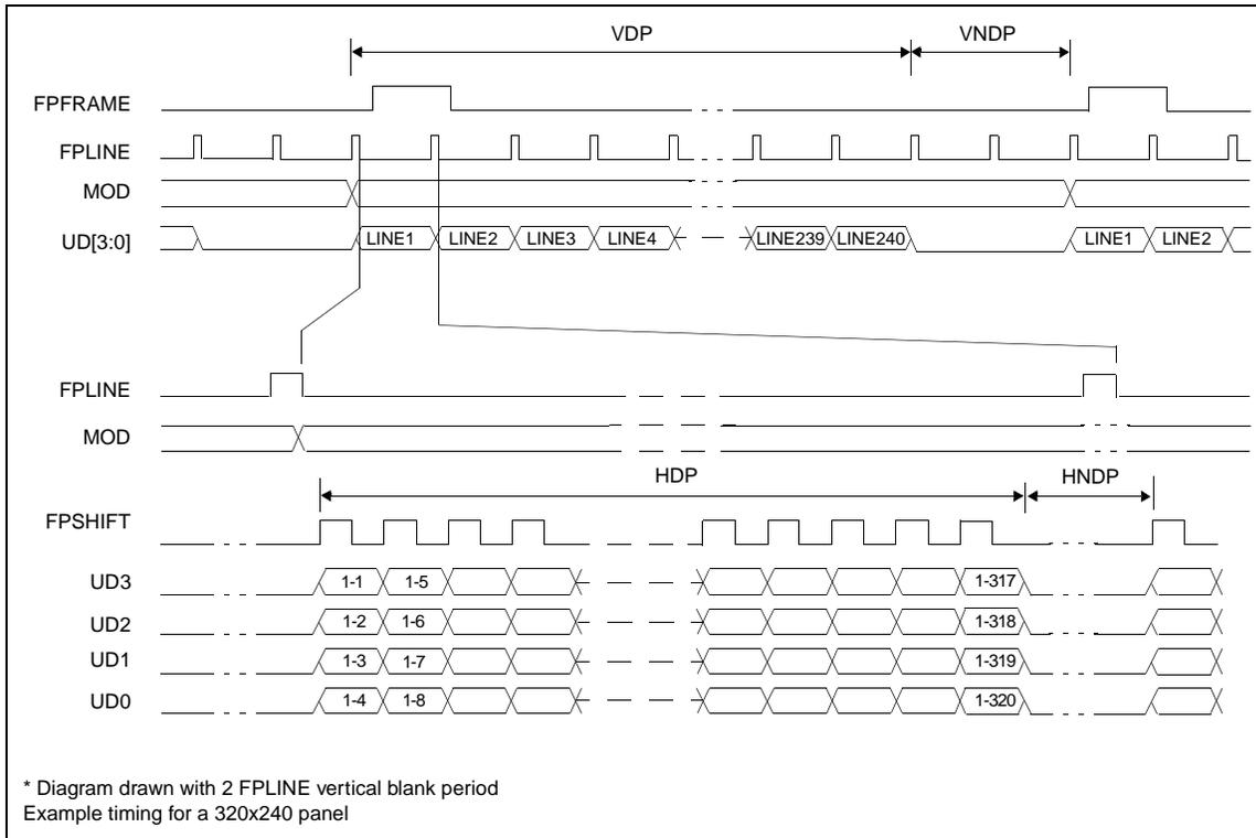
Figure 7-24: 4-Bit Single Monochrome Passive LCD Panel Timing
