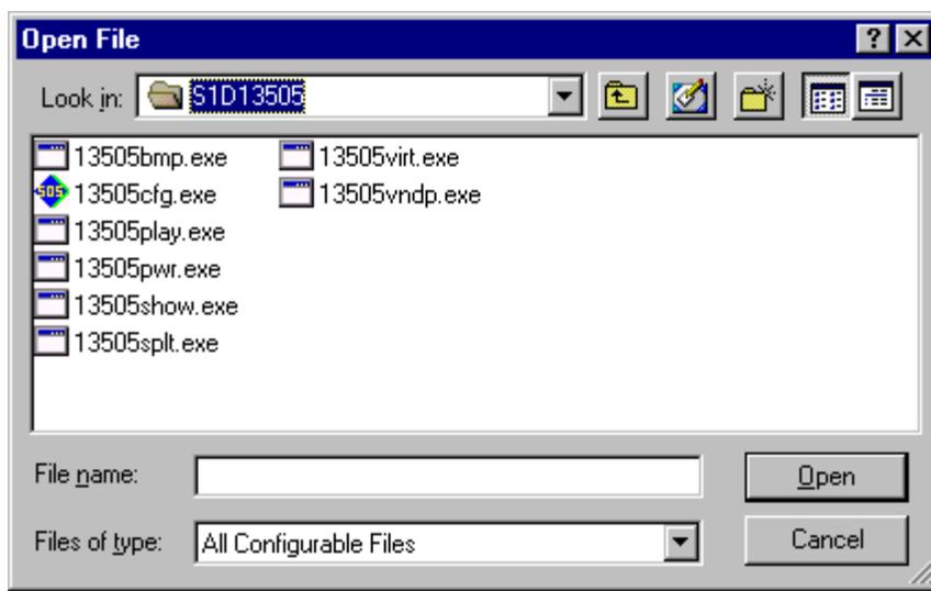
The Open option allows 13505CFG to open files containing HAL configuration information. When 13505CFG opens a file it scans the file for an identification string, and if found, reads the configuration information. This may be used to quickly arrive at a starting point for register configuration. The only requirement is that the file being opened must contain a valid S1D13505 HAL library information block.
