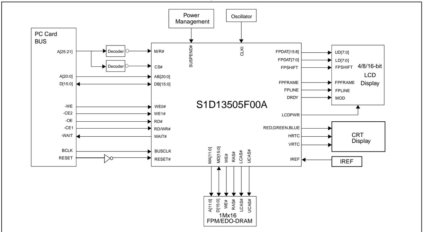
Figure 3-10: Typical System Diagram (PC Card (PCMCIA) Bus)
