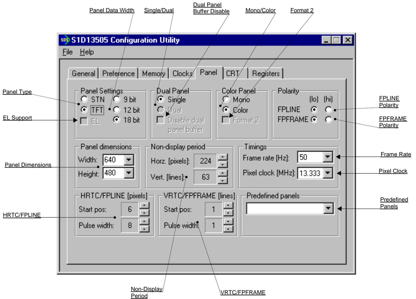
The S1D13505 supports many panel types. This tab allows configuration of most panel settings such as panel dimensions, type and timings.
