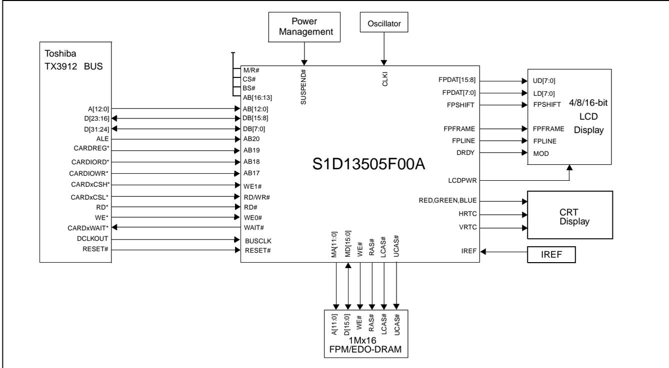
Figure 3-8: Typical System Diagram (Toshiba TX3912 Bus)
