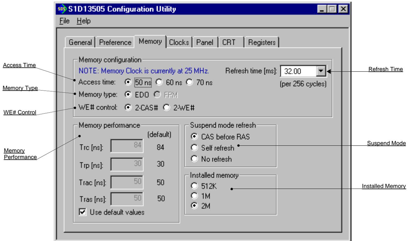
The Memory tab contains settings that control the configuration of the DRAM used for the S1D13505 display buffer.
