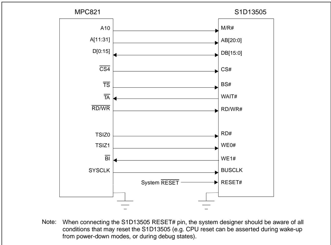
Figure 4-1: Typical Implementation of MPC821 to S1D13505 Interface
