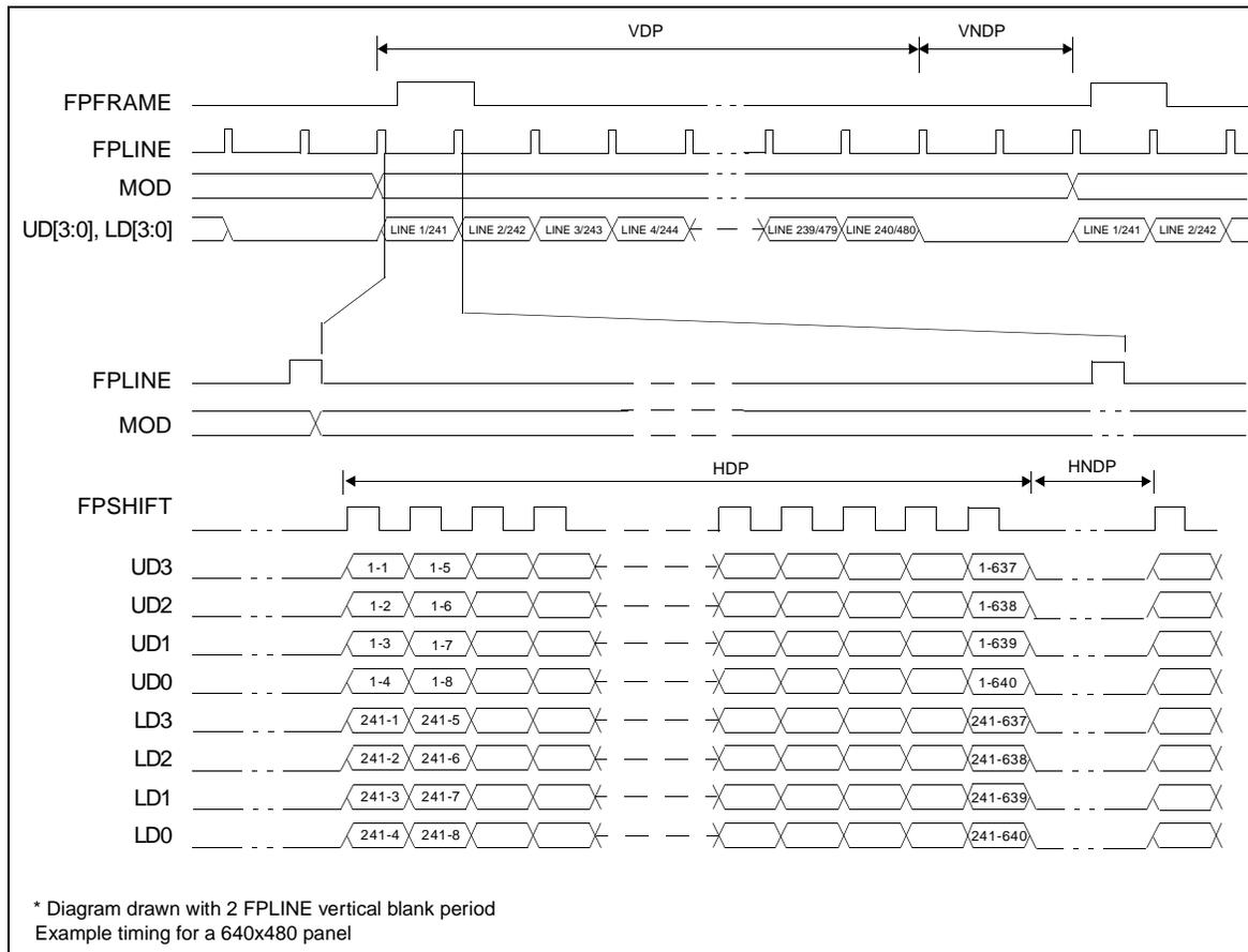
Figure 7-36: 8-Bit Dual Monochrome Passive LCD Panel Timing
