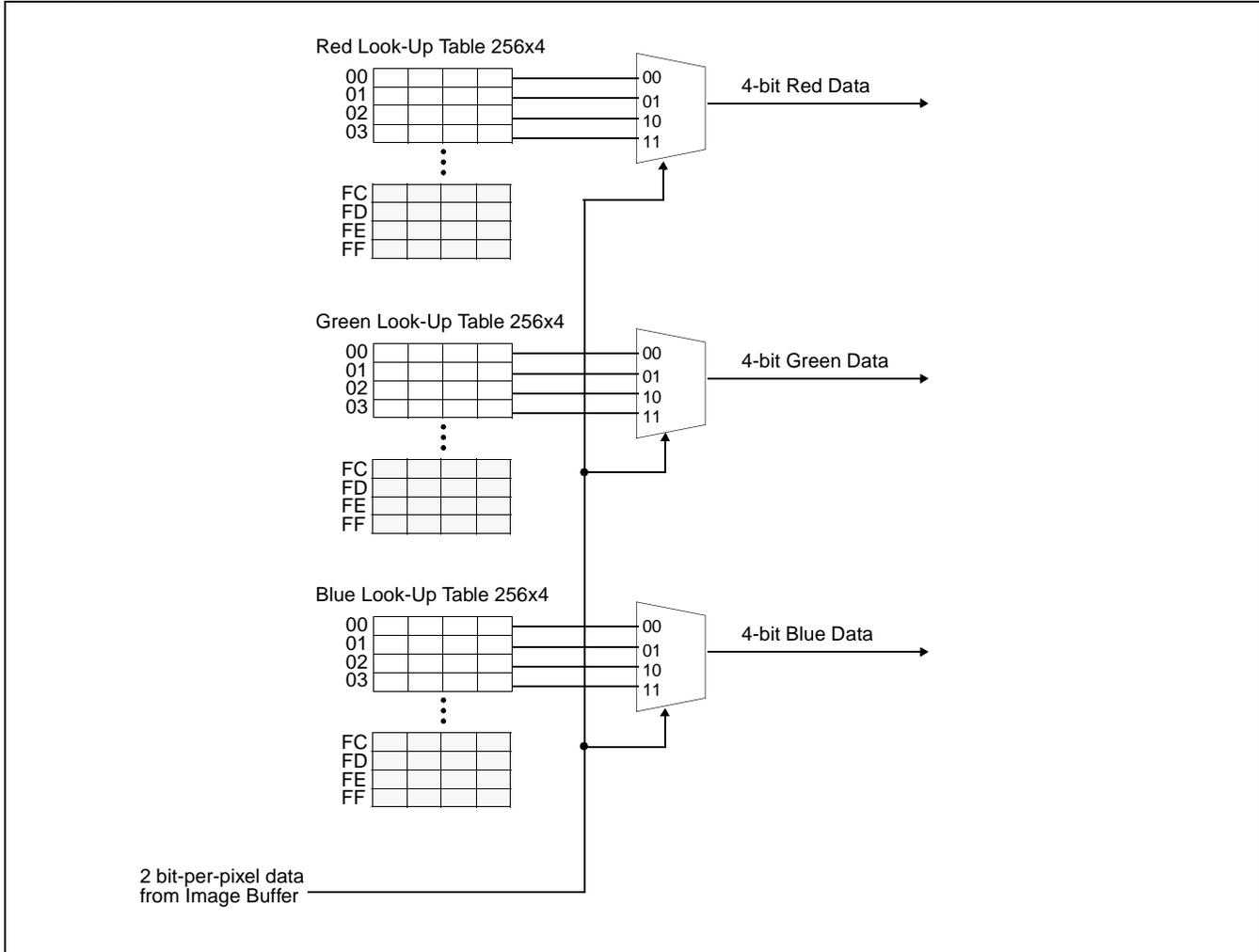
Figure 11-5: 2 Bit-per-pixel Color Mode Data Output Path
