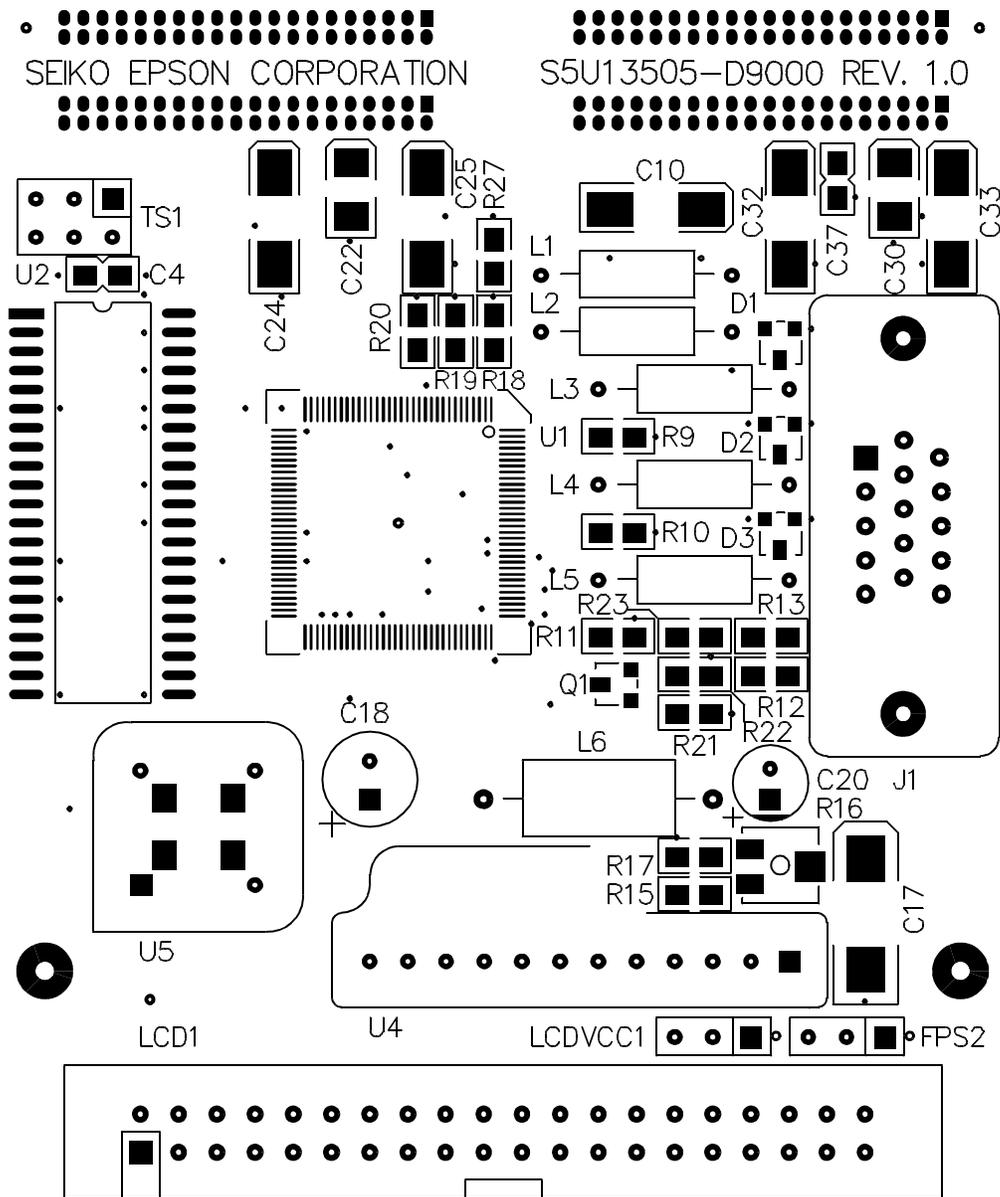
Figure 6-1: Component Placement
