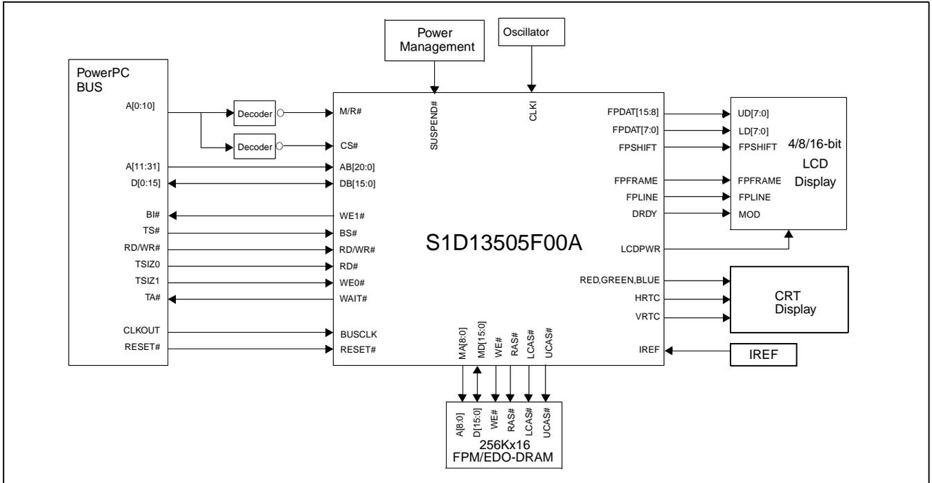
Figure 3-9: Typical System Diagram (Power PC Bus)
