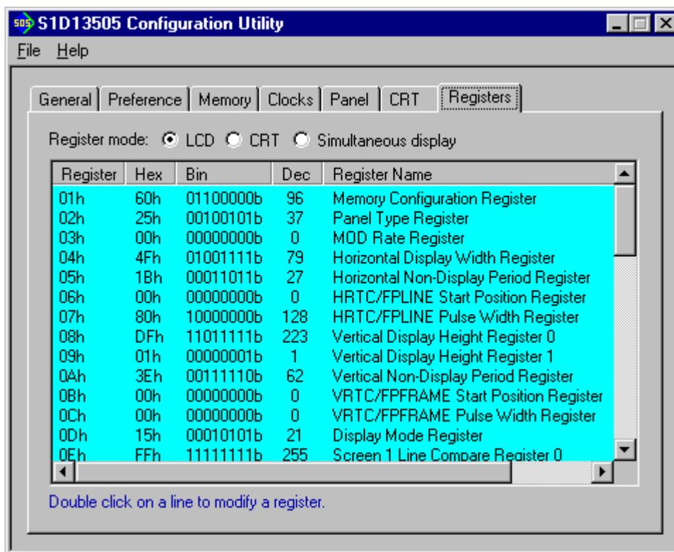
The Registers tab allows viewing and direct editing the S1D13505 register values.
