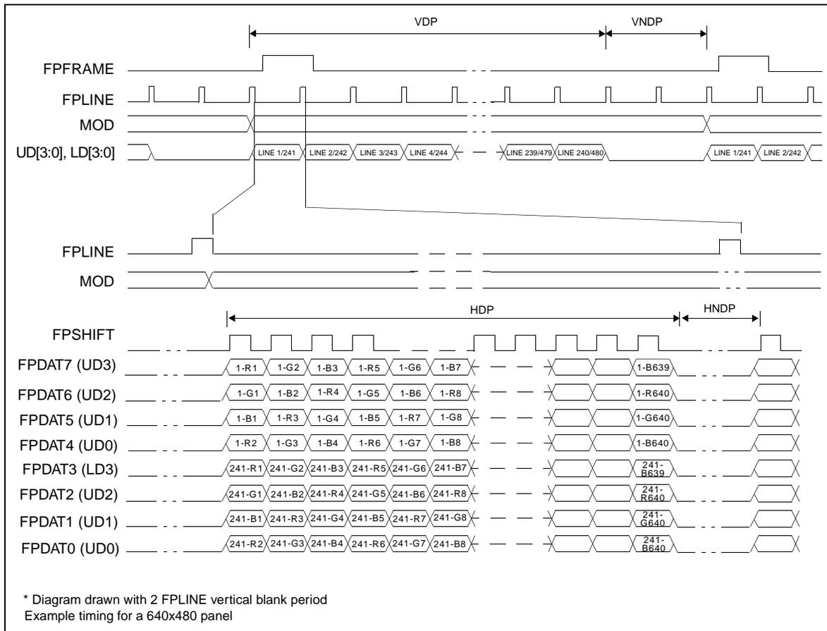
Figure 7-38: 8-Bit Dual Color Passive LCD Panel Timing
