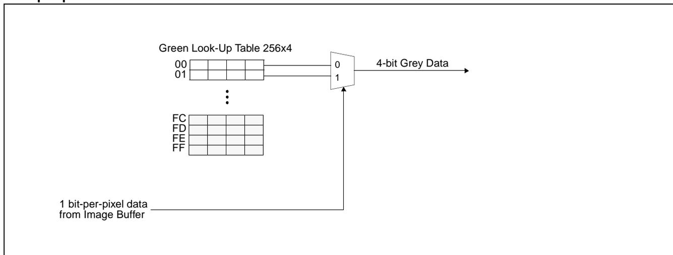
Figure 11-1: 1 Bit-per-pixel Monochrome Mode Data Output Path
