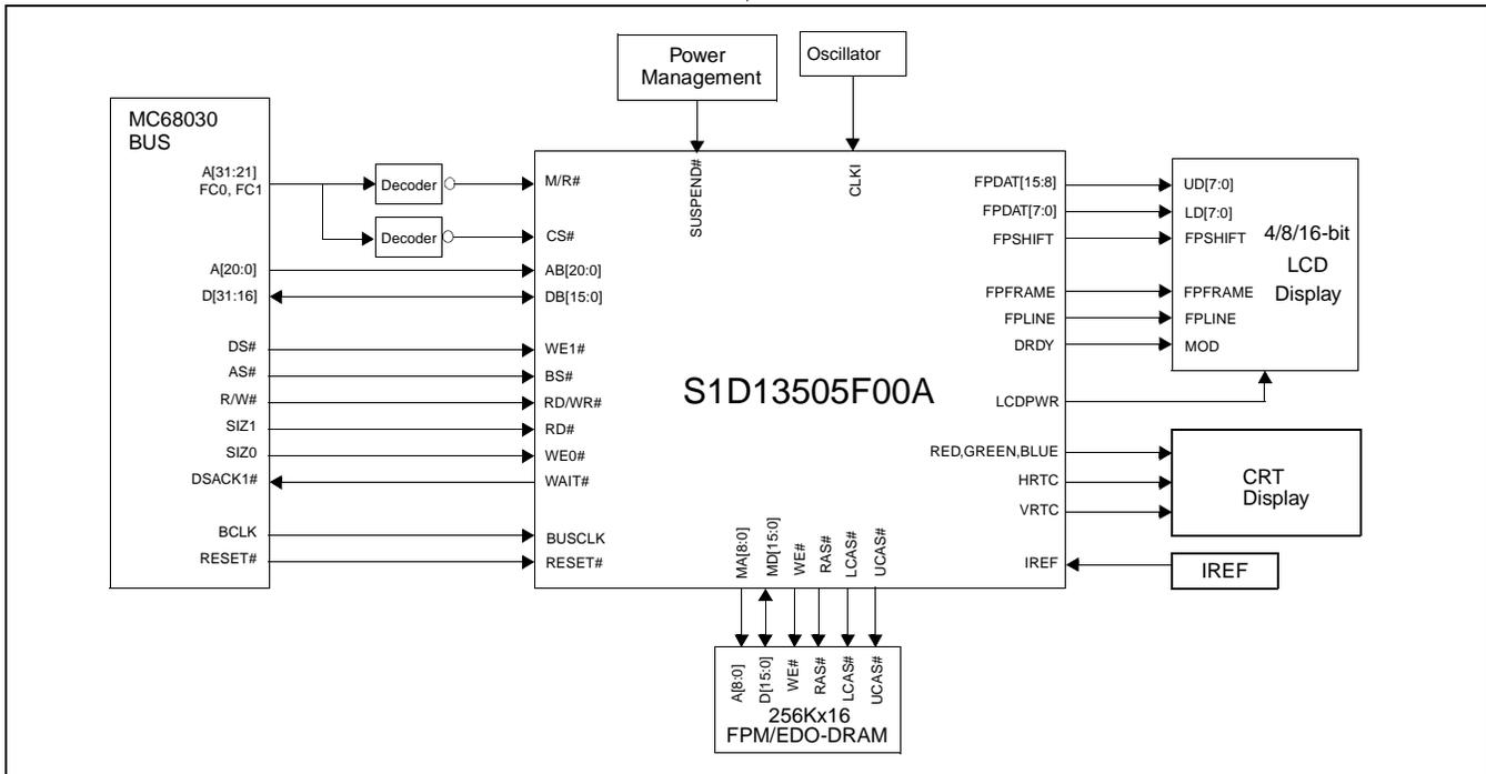
Figure 3-4: Typical System Diagram (MC68K Bus 2, 32-Bit 68030)
