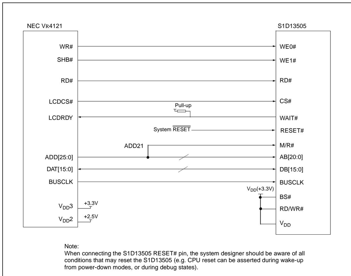
Figure 4-1: NEC VR4121 to S1D13505 Configuration Schematic
