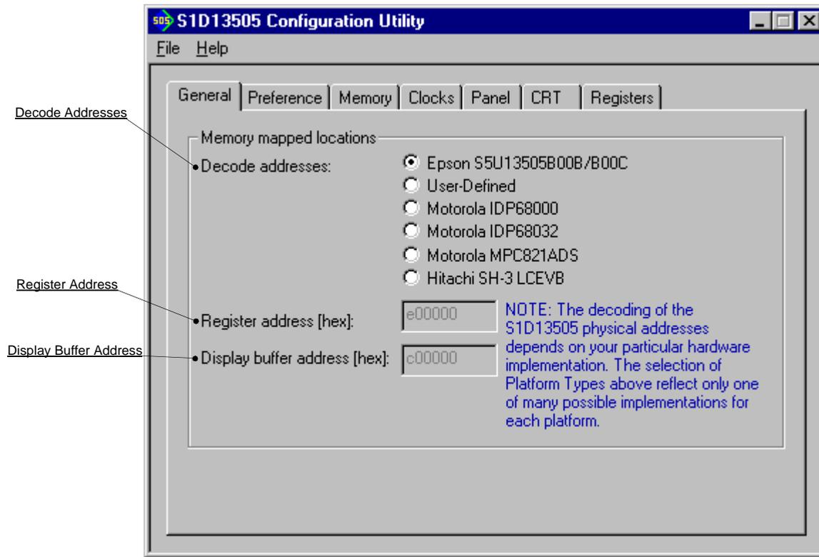
The General tab contains S1D13505 evaluation board specific information. The values presented are used for configuring HAL based executable utilities. The settings on this tab specify where in CPU address space the registers and display buffer are located.
