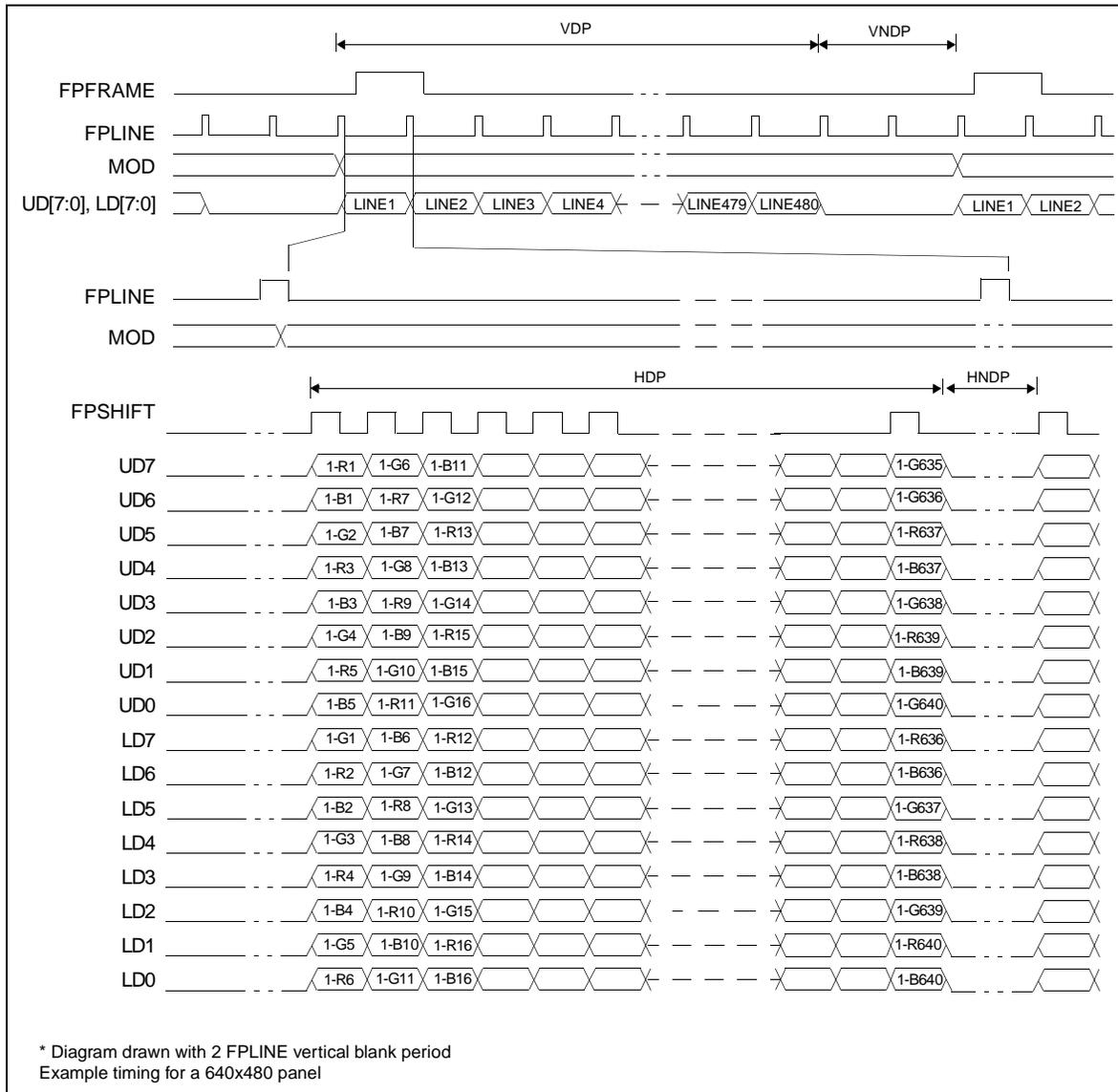
Figure 7-34: 16-Bit Single Color Passive LCD Panel Timing
