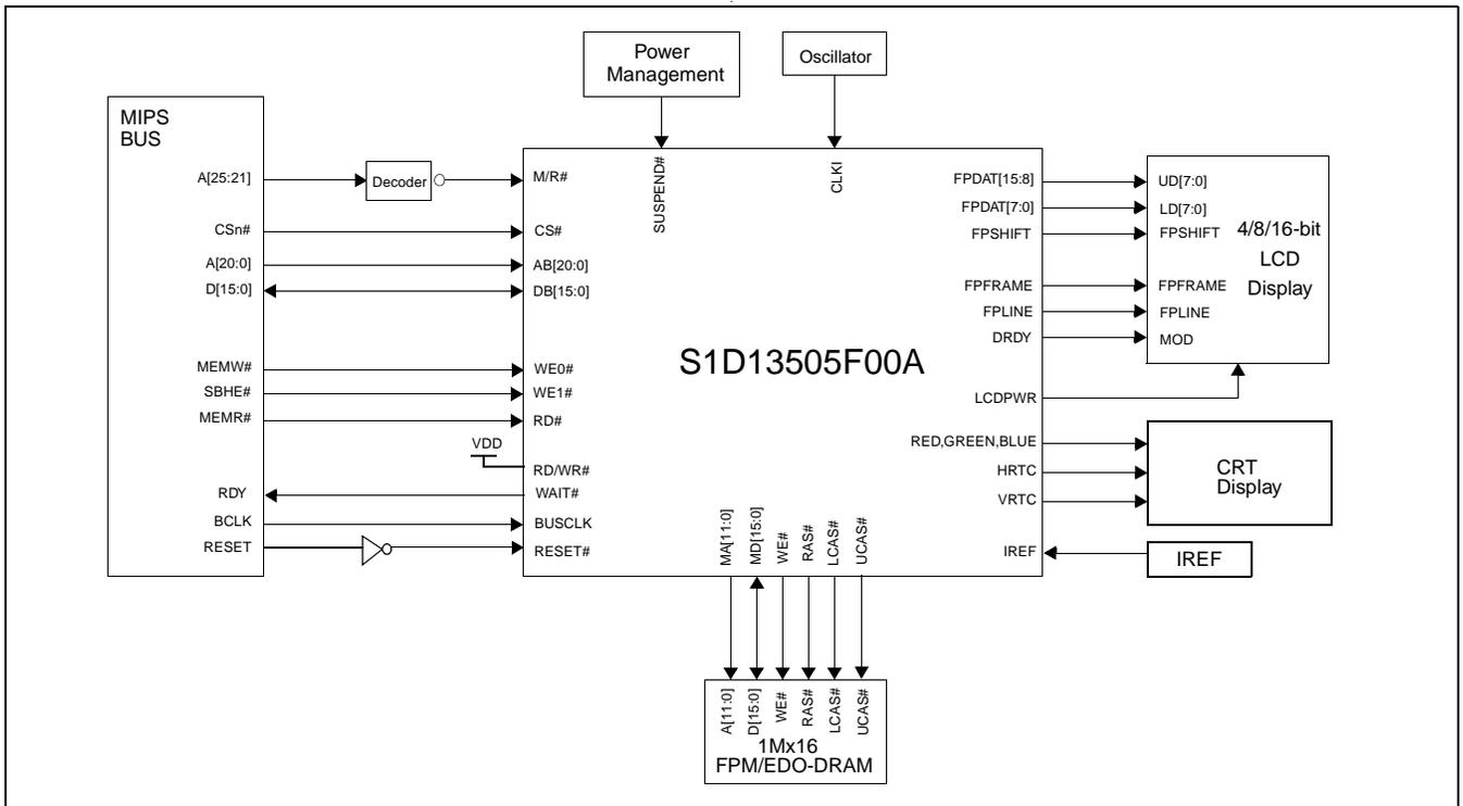
Figure 3-6: Typical System Diagram (NEC VR41xx (MIPS) Bus)
