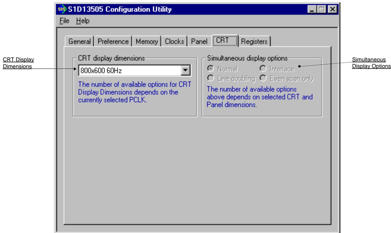
The CRT tab configures settings specific to the CRT display device.
