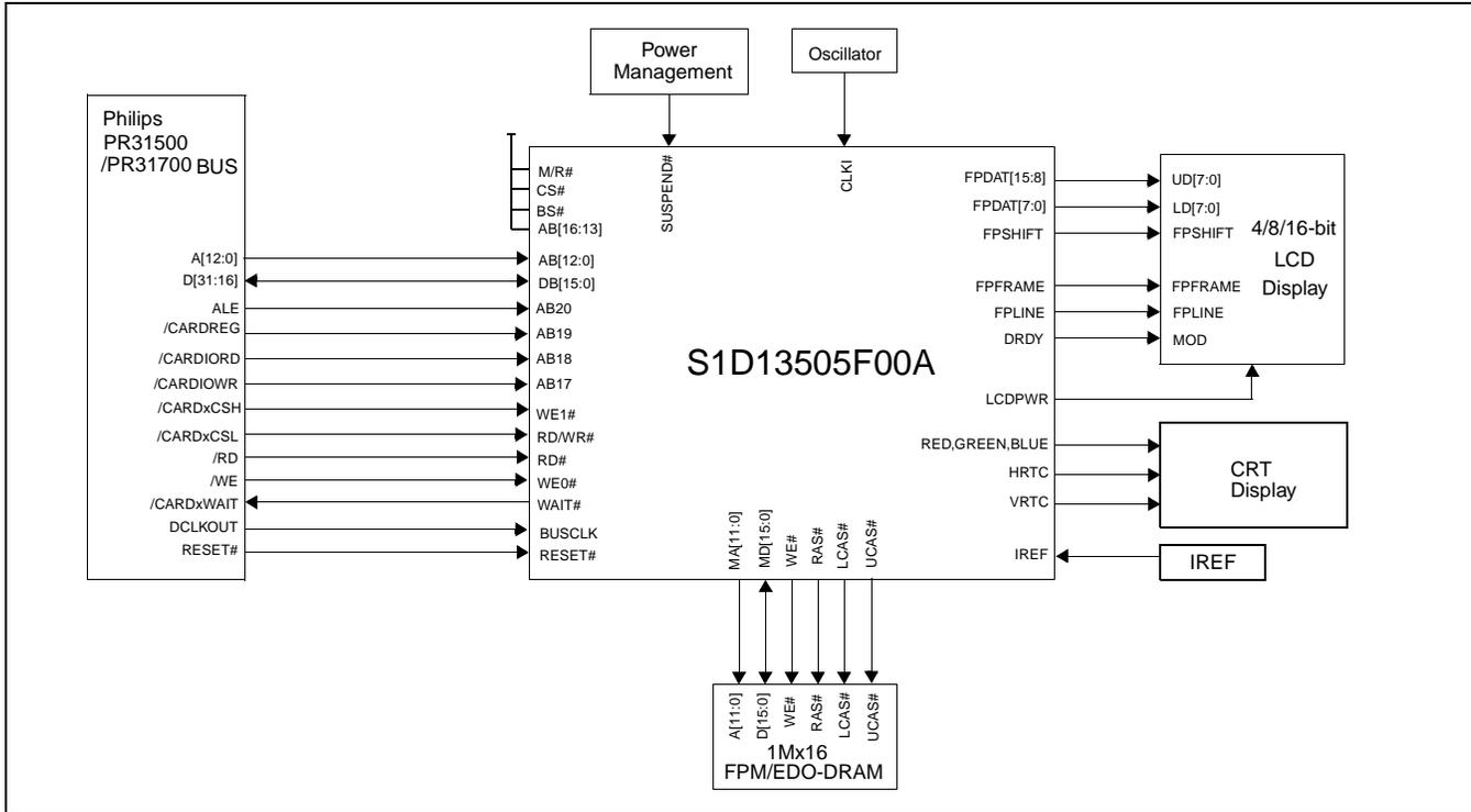
Figure 3-7: Typical System Diagram (Philips PR31500/PR31700 Bus)
