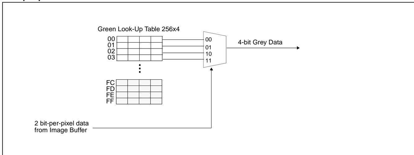
Figure 11-2: 2 Bit-per-pixel Monochrome Mode Data Output Path
