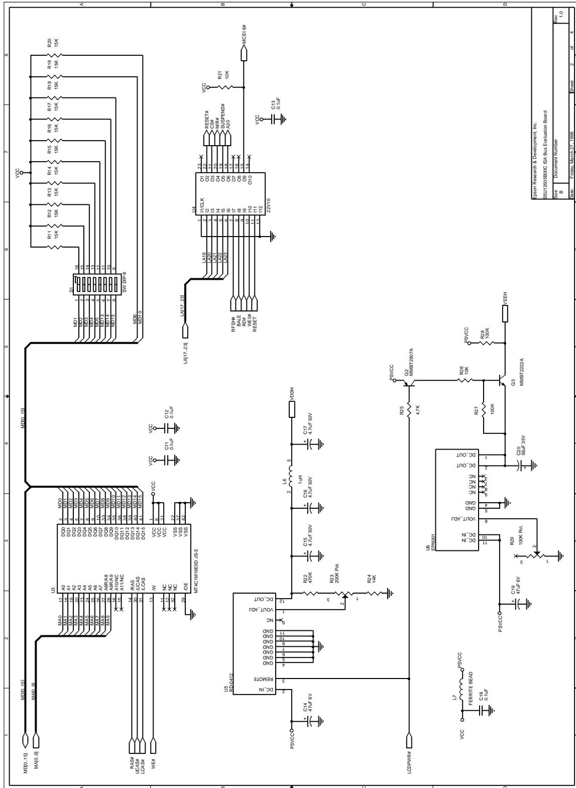
Figure 2: SID13505B00C Schematic Diagram (2 of 4)
