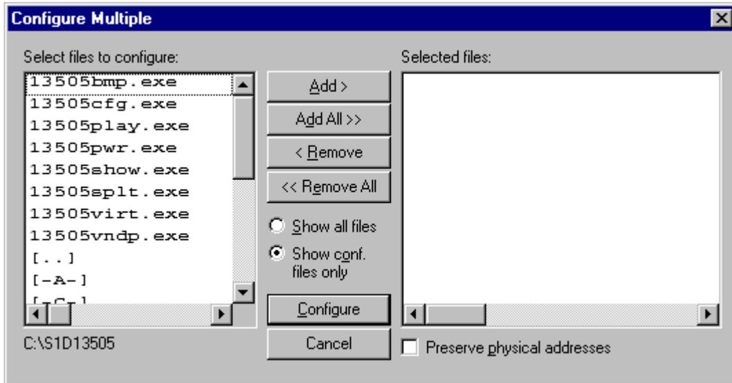
The left pane lists files available for configuration; the right pane lists files that have been selected for configuration. Files can be selected by clicking the “Add” or “Add All” buttons, double clicking any file in the left pane, or by dragging the file(s) from Windows Explorer.
