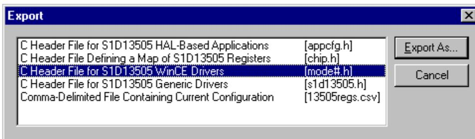
After selecting the file format, click the “Export As...” button to display the file dialog box which allows the user to enter a filename before saving. Before saving the configuration file, clicking the “Preview” button starts Notepad with a copy of the configuration file about to be saved.
