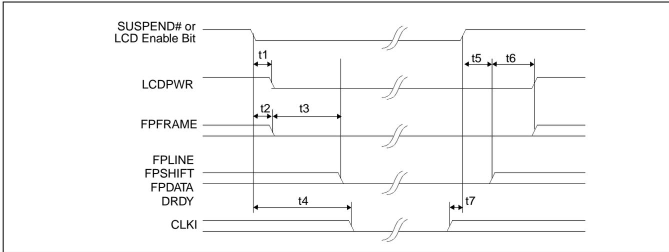
Figure 7-22: LCD Panel Power Off / Power On Timing. Drawn with LCDPWR set to active high polarity
