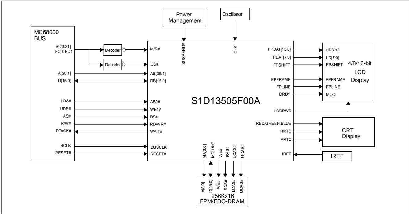
Figure 3-3: Typical System Diagram (MC68K Bus 1, 16-Bit 68000)
