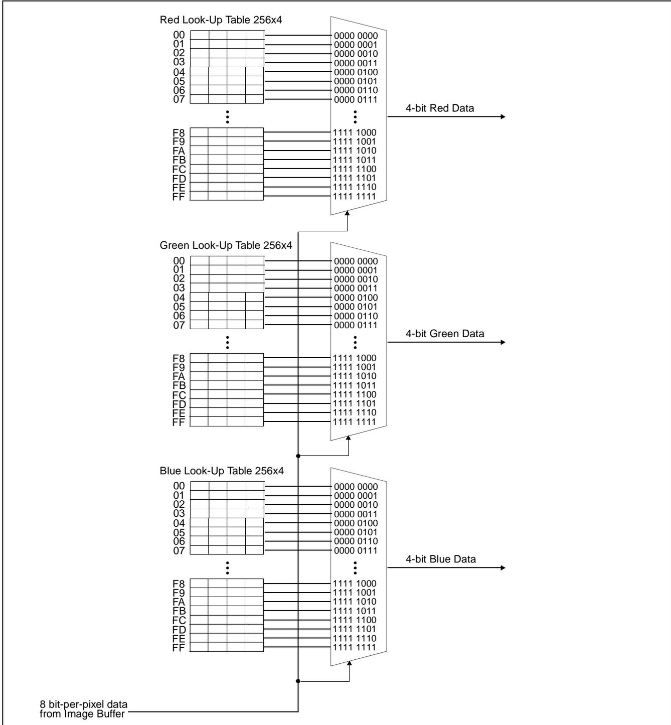
Figure 11-7: 8 Bit-per-pixel Color Mode Data Output Path
