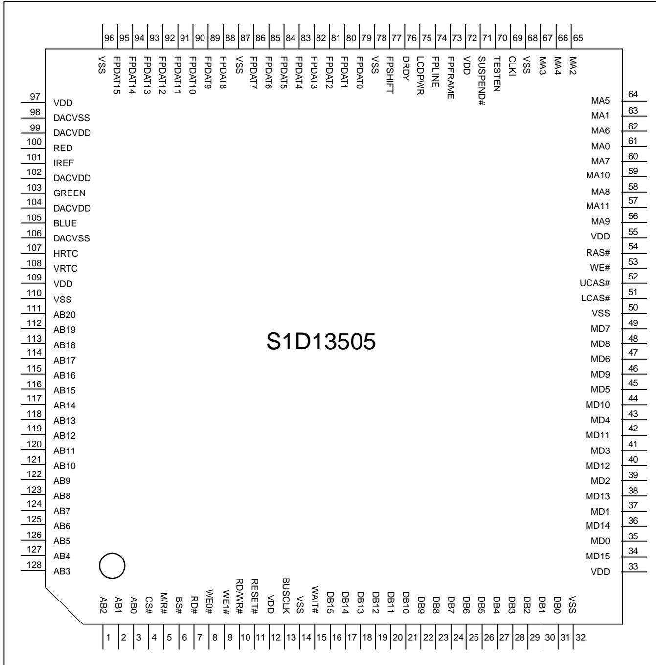
Figure 5-1: Pinout Diagram
