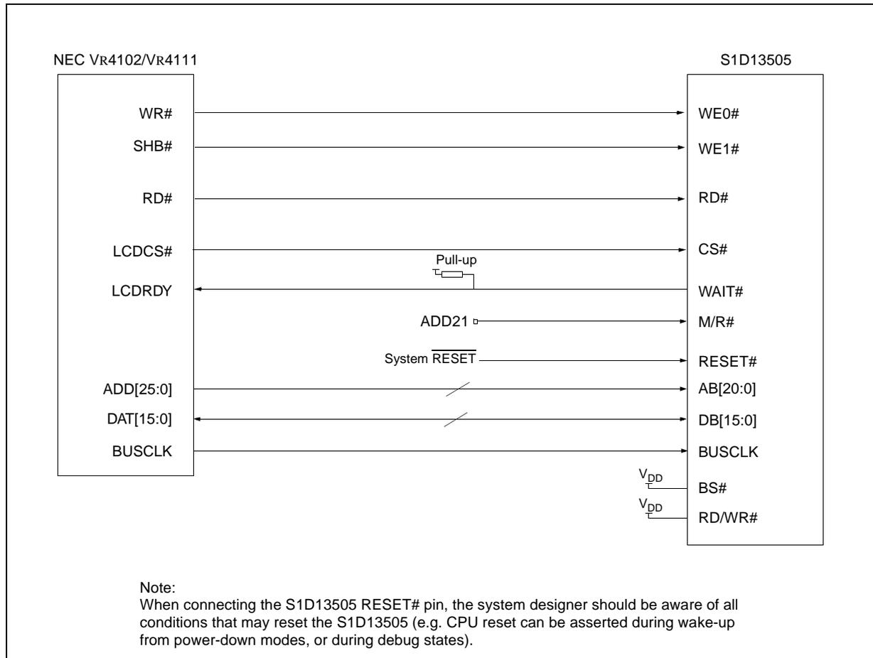
Figure 4-1: NEC VR4102/VR4111 to S1D13505 Configuration Schematic
