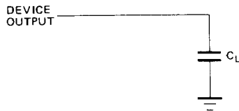
NOTE 9: AC Test Loading on Outputs
