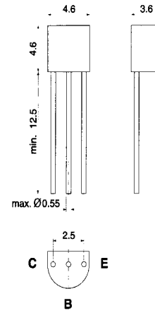
TO-92 Plastic Package Weight approx. 0.18 g Dimensions in mm
