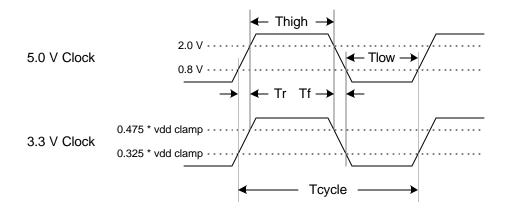
**PCI Clock Specification Timing Characteristics**
