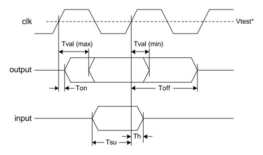
Note: Vtest is 1.5 V in a 5.0 V signaling environment and is 0.4 \* vdd\_clamp in a 3.3 V signaling environment.
