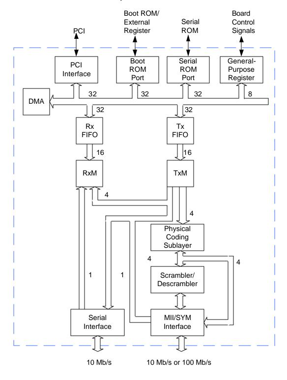
$\label{lower} \textbf{I/O Description} \\ \text{The following section provides a functional description of the I/O pins on the IA21140AF.} \\$
