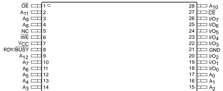
TSOP Package (8mm x 13.4mm) (T13)
